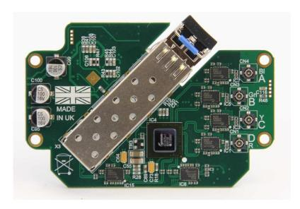
This PCB is ideally suited for use with the popular **CIS 4K Zoom camera** module which has 4x 3G outputs that need combining into a single 12G UHD output. The 4 outputs are synchronised, then combined into 12G, and converted into a fibre optic output. This output can be routed via a Fibre Optic Rotating Joint (FORJ) for 360 deg. PTZs then sent up to 10km to be decoded into a standard 12G SDI signal.
