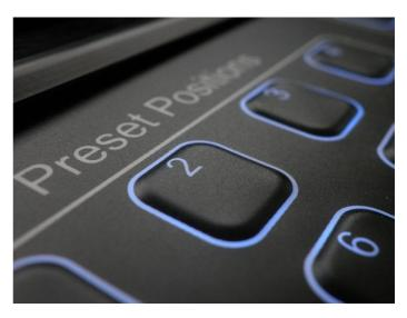
To move to a pre-set position briefly push the button required. If the remote head is programmed to do a profile move to a position this will action the profile move. To move the head quickly to the pre-set position, just push the button again.
